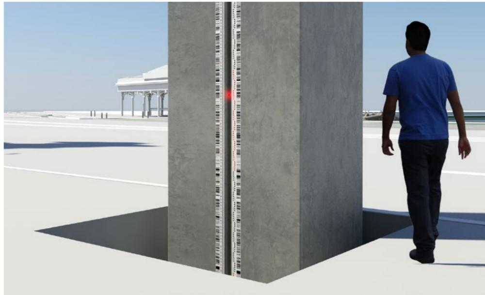
Double seismic column showing sealevel gauge and reveal of underground footing
