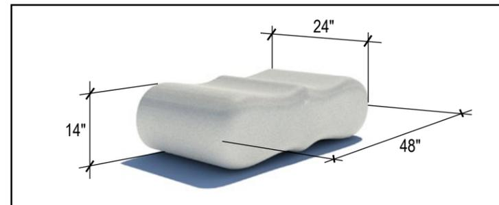
Dimensions of both the **Stone SeaRisers** and **Concrete/Rubble SeaRisers**
