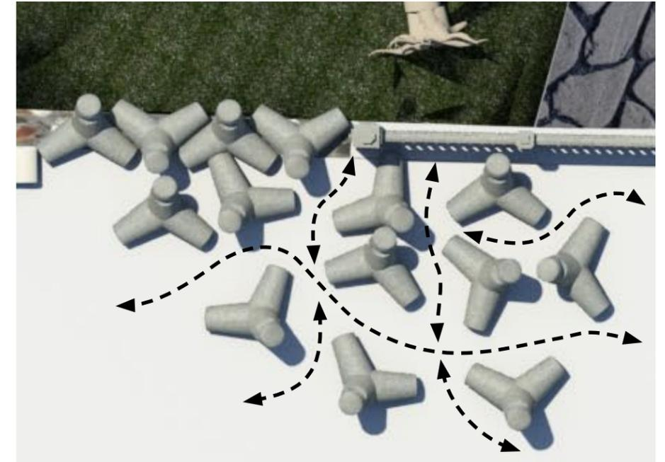
Plan view showing pedestrian flow spacing of dolos
