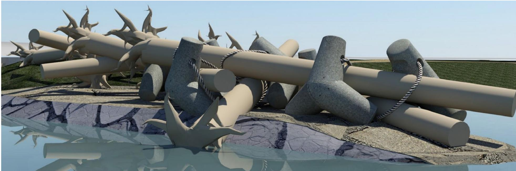
Proposed root wads (concrete anchor version)
