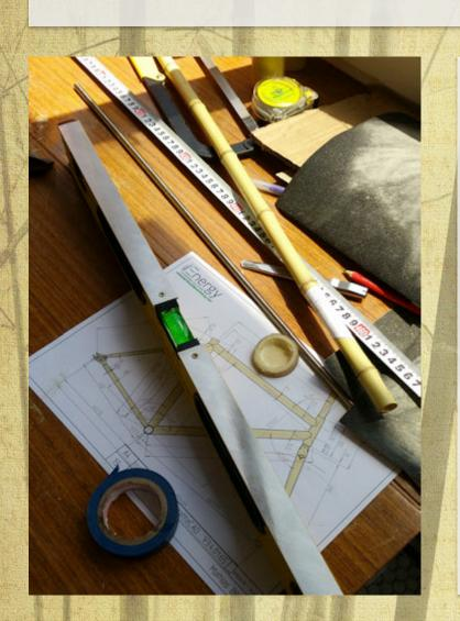
Slightly more advanced type of workshop where participants gets to build their own bamboo bicycle frames starts with using bicycle CAD tool to design the frame and goes on by choosing right bamboo tubes, cutting them to right dimensions, sanding down, and fitting them on the jig before they finally get to be wrapped with carbon fiber and glued with epoxy. Final product is usable bicycle frame.
